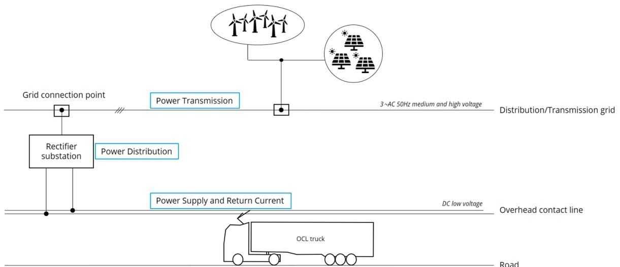
Figure 2 Schematic representation of the power supply of the eHighway ([Werner 2020] according to [Biesenack et al. 2006])
