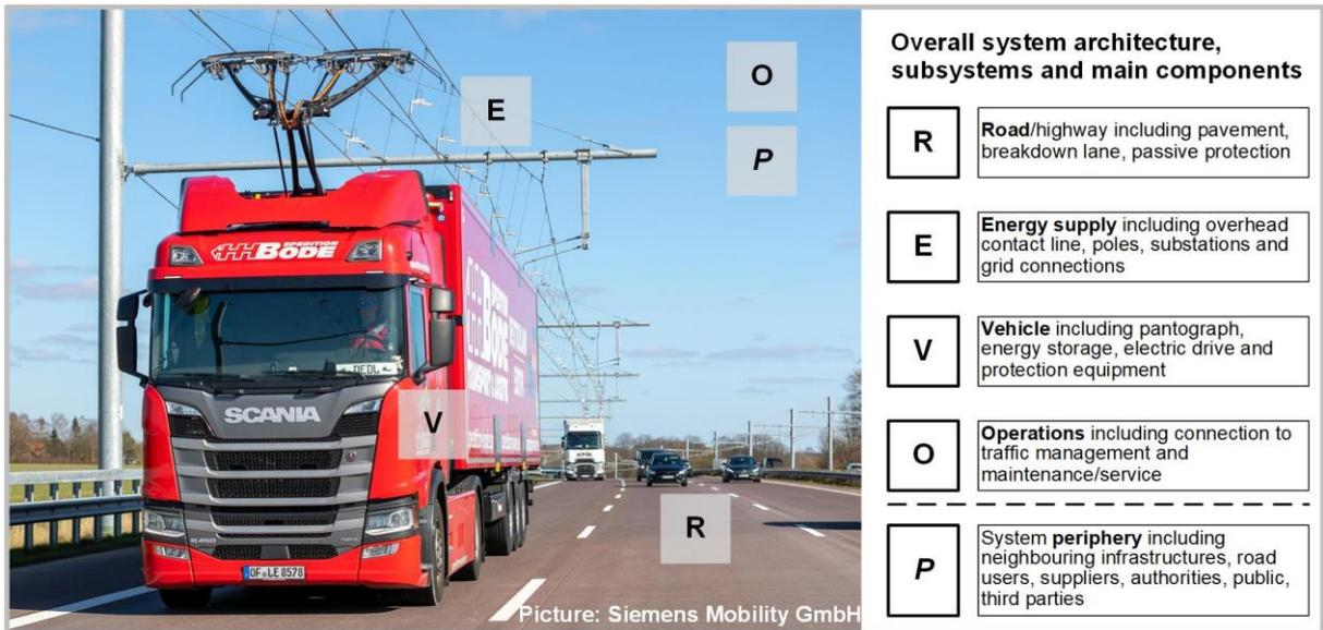
Figure 1: Overall system architecture and subsystems of the overhead contact line truck system (Image source: Siemens Mobility GmbH with additions by the author)
