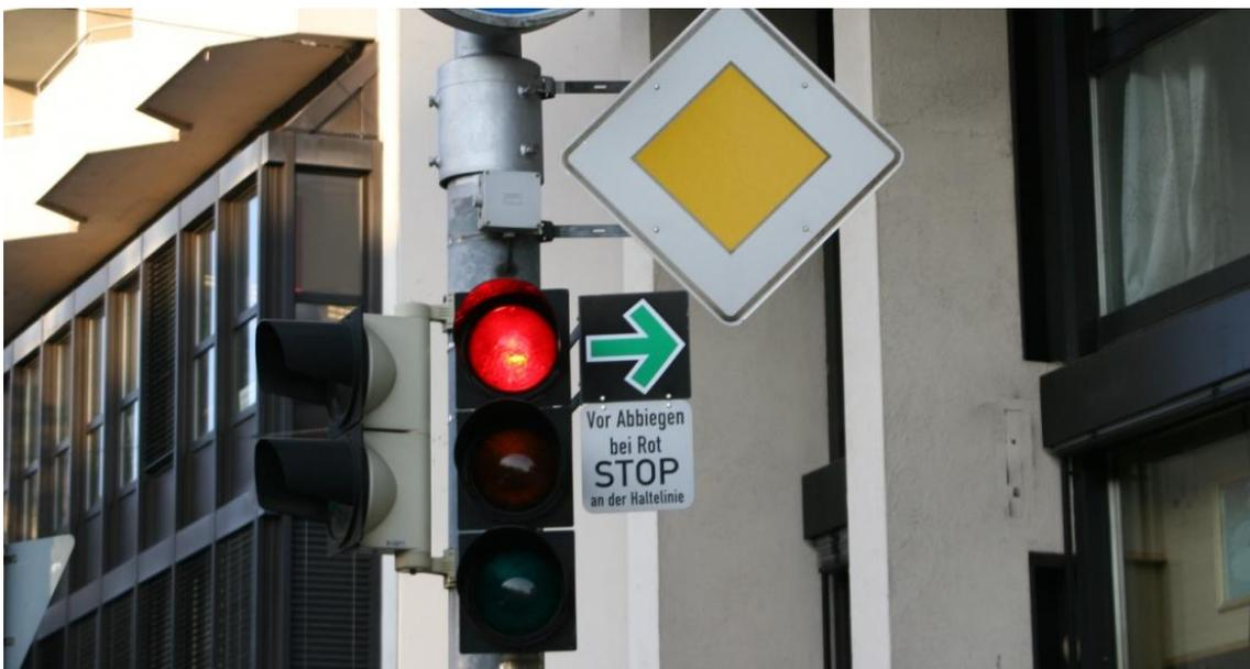
Figure 2 – Static green arrow sign in Germany (Source: TU Darmstadt, Chair of Transport Planning and Traffic Engineering)
