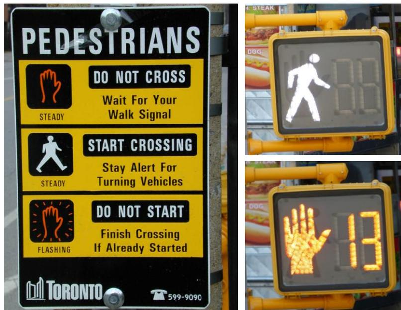
Figure 4 – Rules for using traffic lights for pedestrians and displaying remaining time for pedestrians in North America (Source: TU Darmstadt, Chair of Transport Planning and Traffic Engineering)
