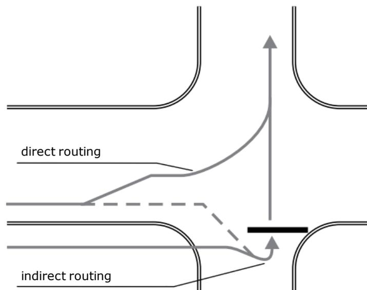
Figure 7 – Direct and indirect routing of left-turning bicycles at intersections (Source: FGSV, 2010b)
