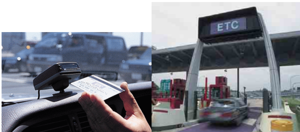
Picture 8: Ob-board equipment with IC card and example of ETC in operation [HIDO 2001]
